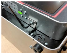
Remove Allen bolt from base of controller.
