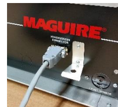
Secure Remote Mount Base cable to Blender Controller.
