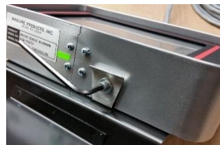
Hang controller on Remote Mount Base and secure Allen bolt to controller.
